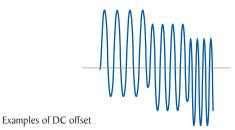
The 9830 Series is capable of generating AC+DC waveforms. When operating in pulse, step and list mode, the AC signal can be combined with either a positive or negative DC offset voltage, allowing users to create a wide range of waveforms.
